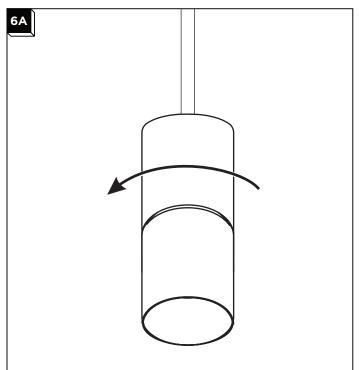
**1** For adjustable and wall wash fixtures: the cylinder can rotate 358° to assist with aiming at the wall.
