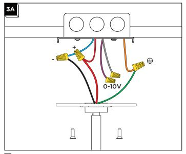
1 Use the following wiring diagram to wire your fixture.
