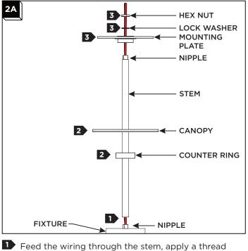
Feed the wiring through the stem, apply a thread lock adhesive to the threads, and screw the stem to the top of the fixture until flush (**do not over tighten**).
